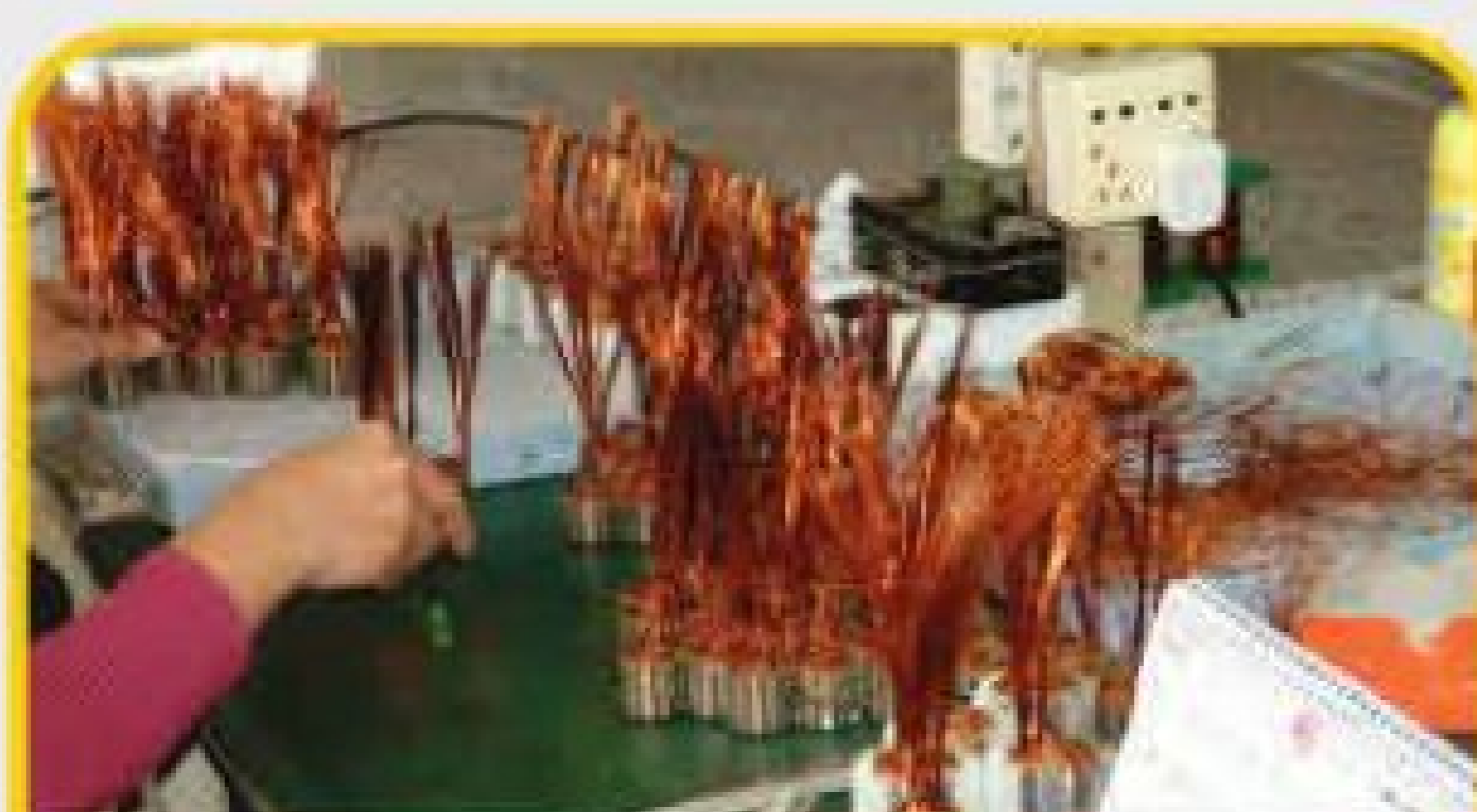
Wound stators having the leads trimmed and prepped for soldering on the bullet connectors.
