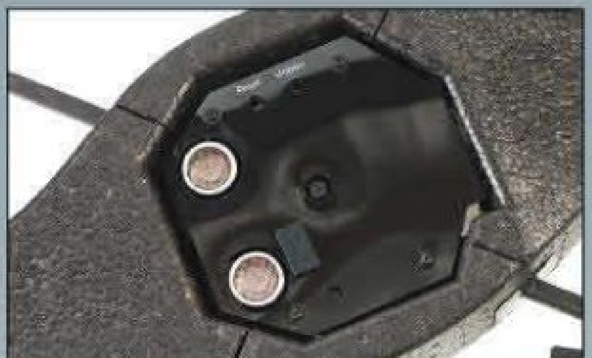
The bottom of the AR. Drone houses a high speed camera, ultra sound altimeter and a USB plug.
