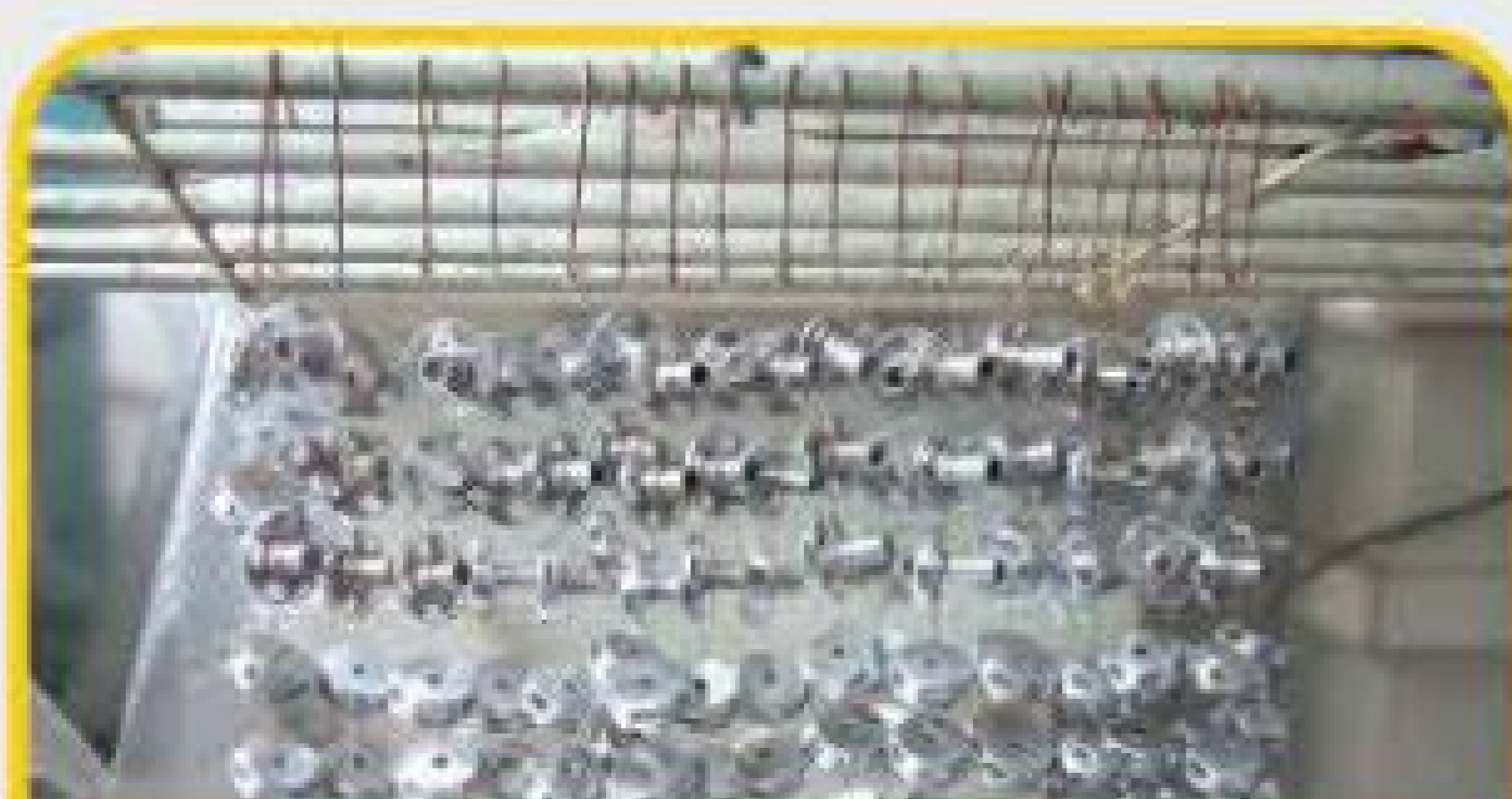
Bearing tubes and fan assemblies for HK-4025 motors being prepped for plating.
