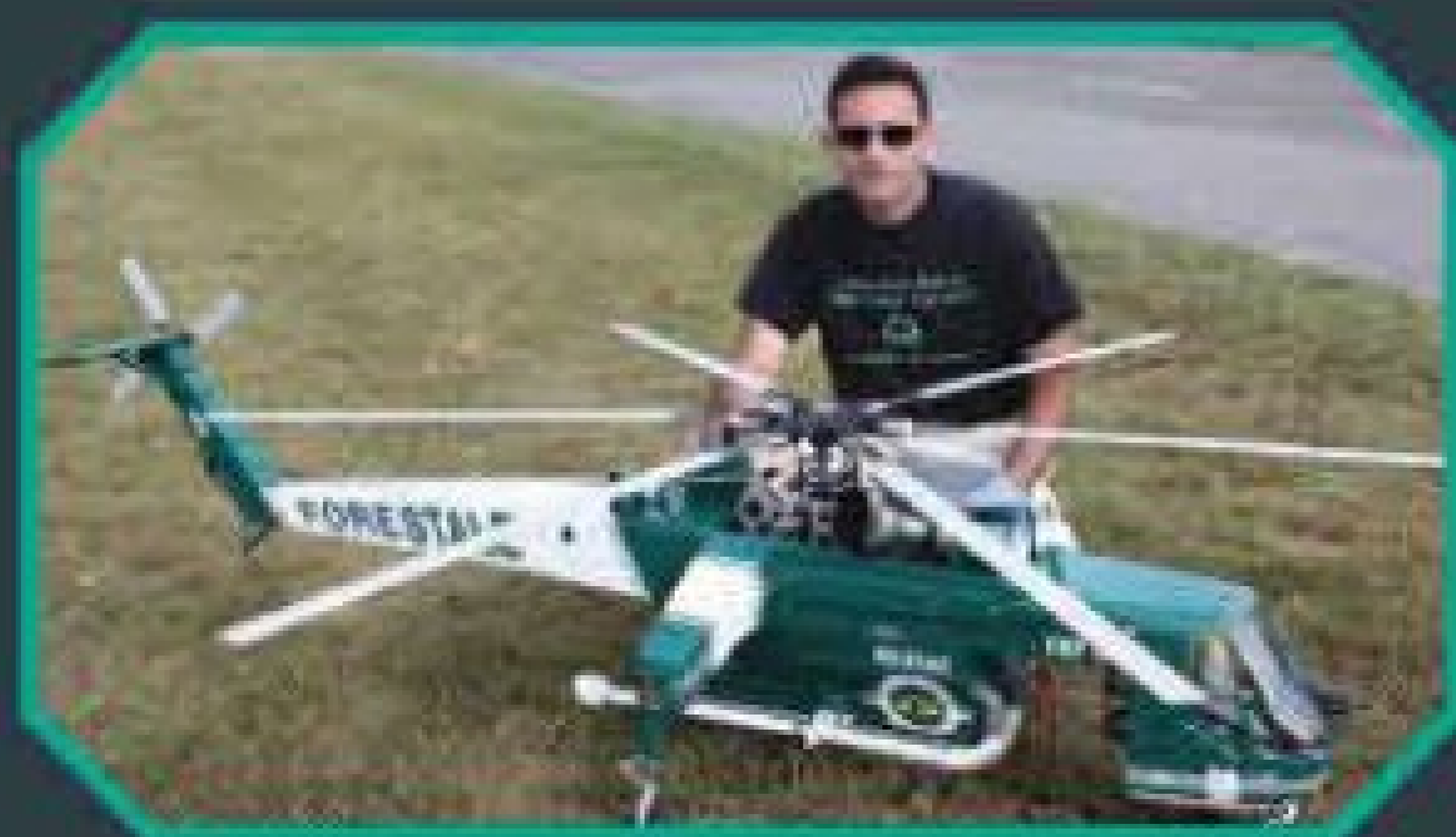
Joel Rosenzweig, Boston, MA—Vario Sikorsky S-64 Skycrane, home built electric conversion, Vario 6 blade head with 1000mm blades.
