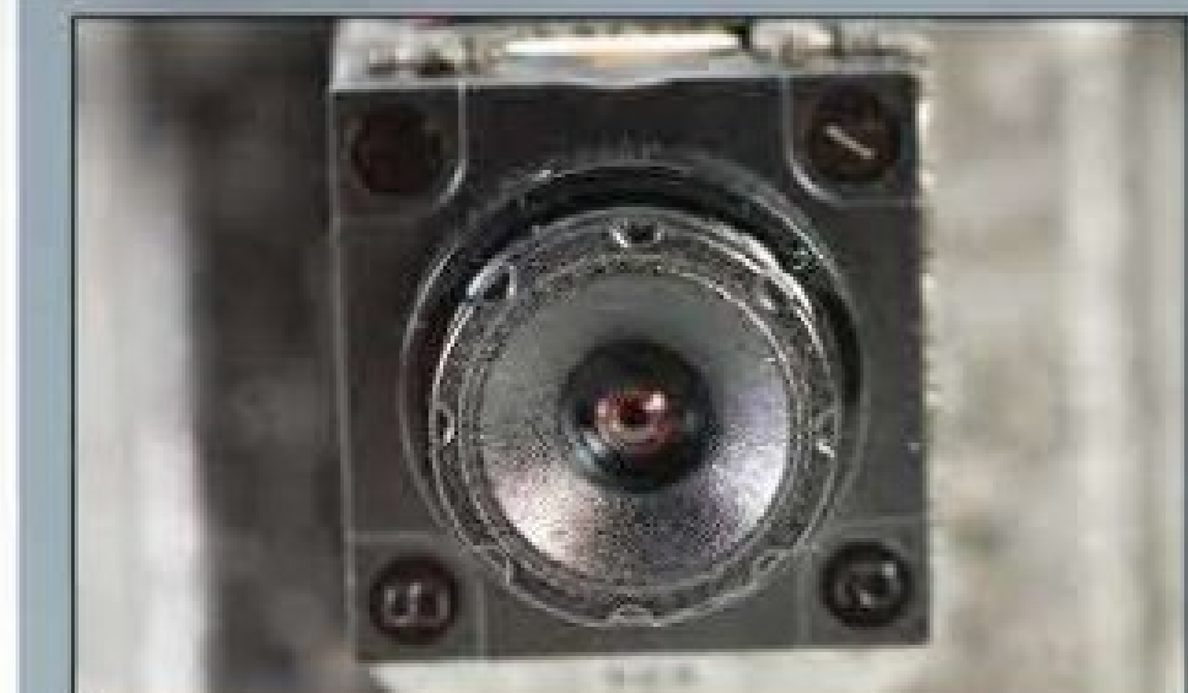
The front camera has a resolution of 640x480, and a frame rate at 15fps.
