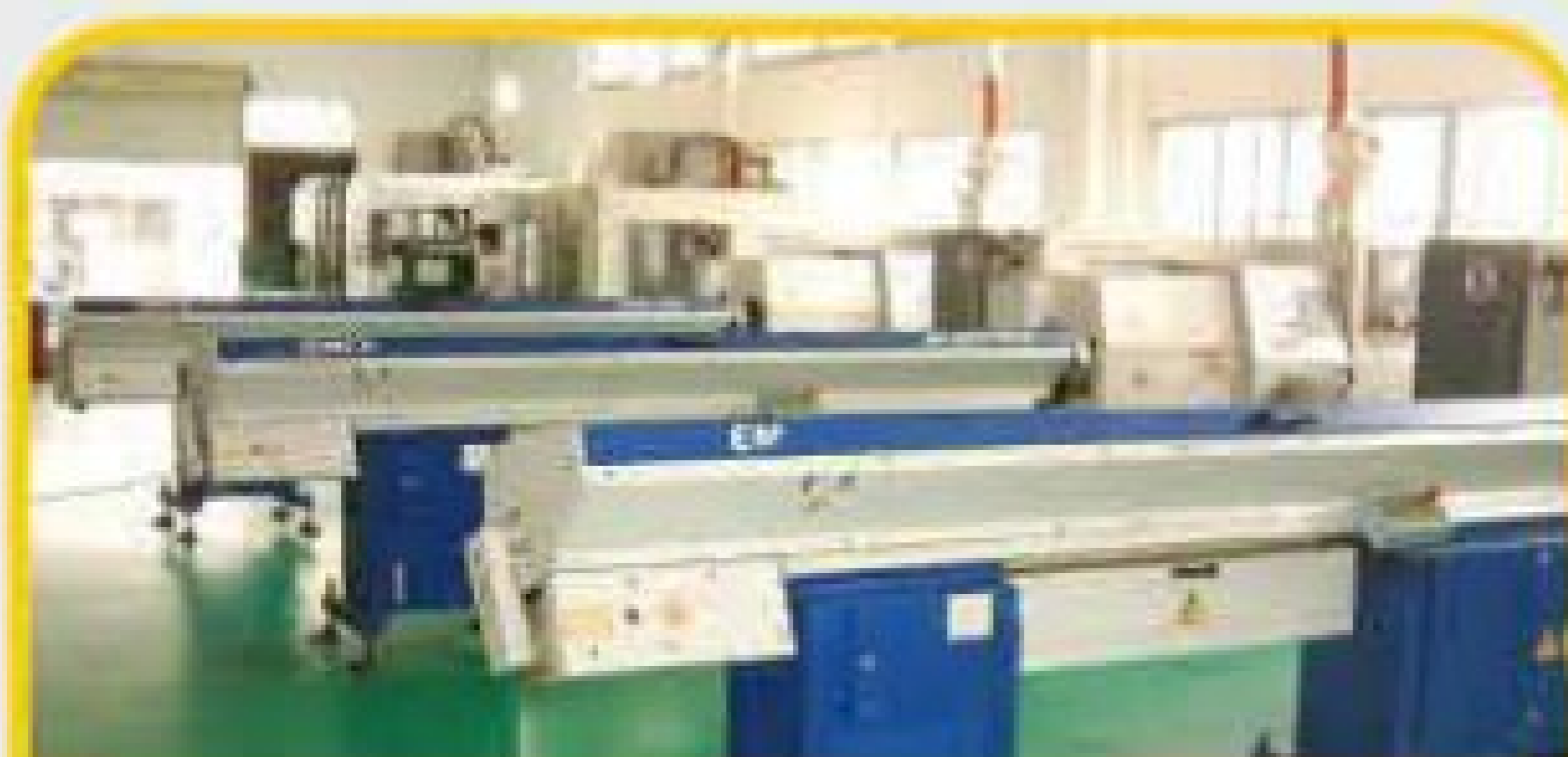
Three auto-feed CNC lathes where many of the motor parts are made. Two workstation machines can be seen in the background of this photo.
