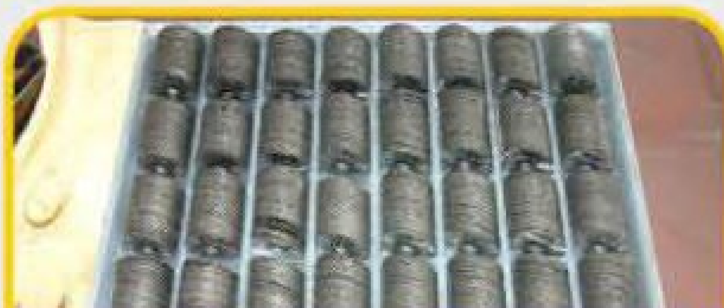
Scorpion makes all of their own stators. Here are stacks of individual laminations after they have been punched, on the way to the press where they will be assembled into stators.
