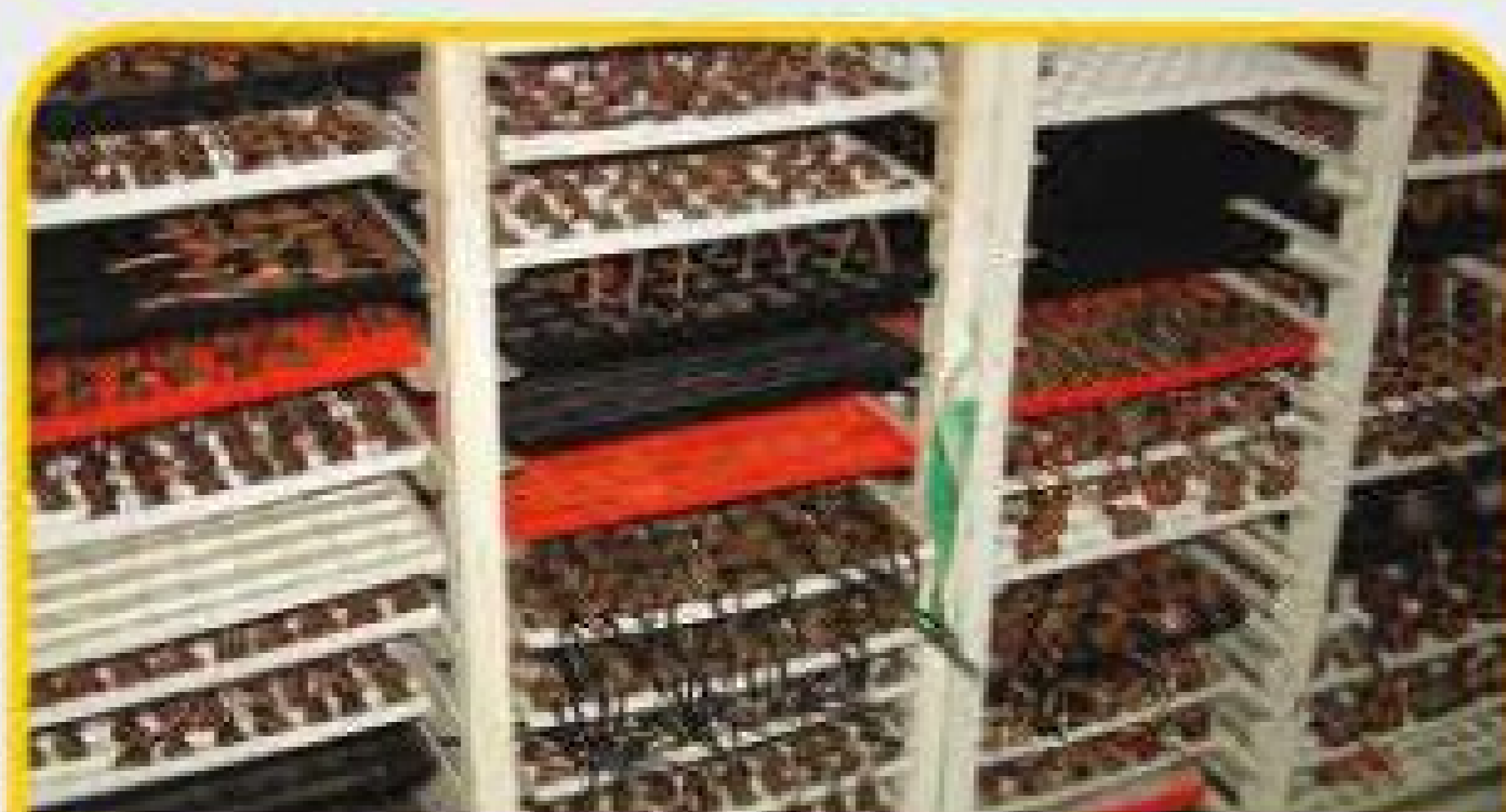
Trays of completed stators, ready to go to final assembly.
