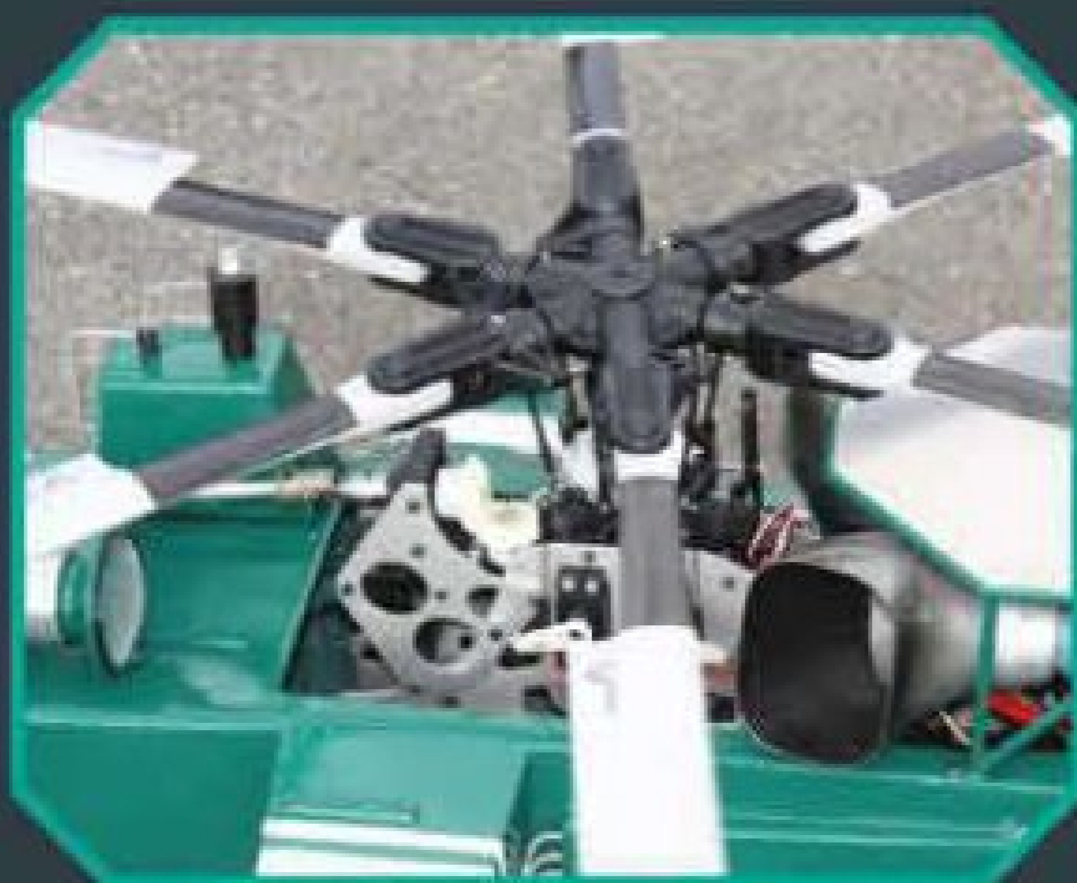
Joel Rosenzweig, Boston, MA—Vario Sikorsky S-64 Skycrane, home built electric conversion, Vario 6 blade head with 1000mm blades.
